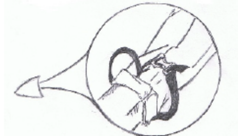
Detail of inflation tube on blower. Blower runs continuously.
